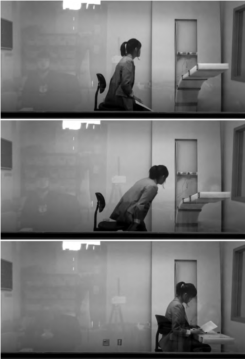
Figure 3.8.3 A robot surface for writing: still images taken from the video of the lab study. (Consent was collected from participants to publish their likeness as per Cornell University IRB approval.)
