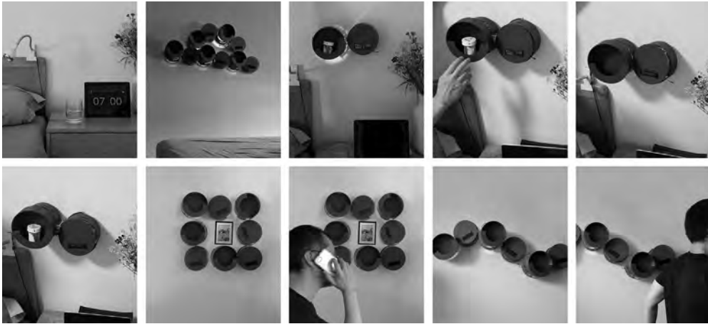
Figure 3.8.2 SORT, delivering a medication bottle to a user at a scheduled time and offering nonverbal reminders.
